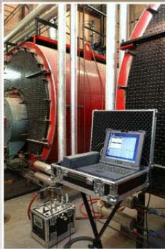
Equipment for testing safety-valves during production, at right temperature and pressure. The test results shows directly in graphic.
